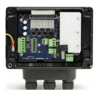
Leak Alert 75 showing external keypad (option) and internal kepad
